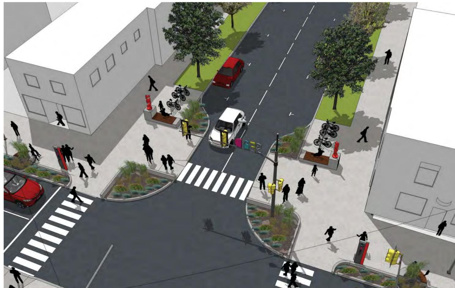
Typical street dimensions as shown in the current plan show 12' wide drive lanes on primary arteries with 10' drive lanes on secondary feeder streets. The parking lanes on each side for both street types are both 8' wide. Standard 24" curb and gutter sections will be used throughout with the added consideration for the stormwater access to the bio-filtration planters.
